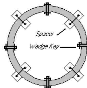
is economical in its use of cement, and makes it possible for a man to dig within the ring should the well require deepening at a later stage. The 600 mm ring is too small for a man to operate a pick.
