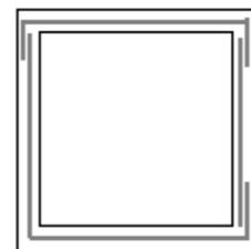
**For water tank floor:** we do not know exactly in which direction the curb will be. So the iron bars will be in the middle of the section and special care is given to the corner.
