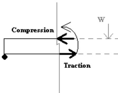
Let's consider now the section of the beam. Appear on it a moment M and practically on this section this moment could be describe by to yield: a traction and a compression.
