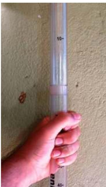
2) Hold the tube vertically (hold the lower tube!) and pour the water sample into the tube until the marker just disappears when viewed from the top of the tube. Avoid creating bubbles, as these may cause false reading. Do not strain to see the black circle as this can sometimes cause biased results.
