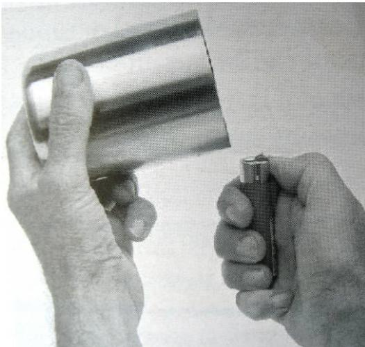
2) Carefully ignite the methanol in the sample cup. Allow the methanol to burn for several seconds.
