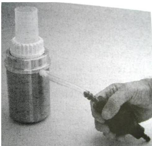
6) Connect the vacuum pump with the filtration base. Squeeze the pump to draw all the water through the filter. Stop pumping once the water has gone.
