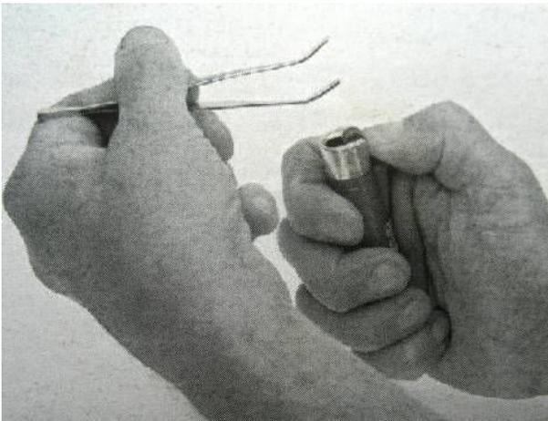
3) Flame the tips of the tweezers with lighter for 5 seconds and leave to cool. Keep it away from any contacts on any surface, hands or tool....
