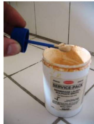
3) If you want to verify the weigh, put those 8 spoons of Lauryl Sulphate powder on a piece of paper. Switch on the balance and weigh to verify the amount of Lauryl Sulphate. Pour the Lauryl Sulphate in the metal cup into the 50ml of water. Shake it gently to dissolve the powder.
