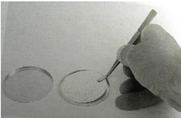
8) Lower the membrane on to and adsorbent pad in a Petri dish.
