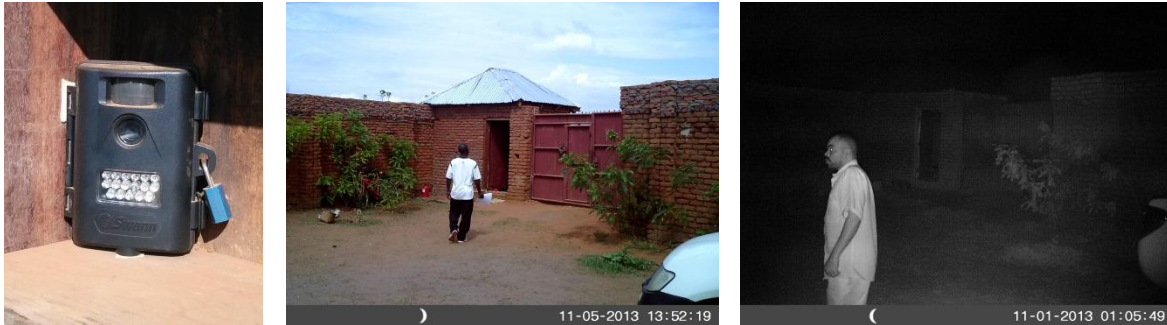
A battery powered security camera with night vision and motion sensor at the Child Health Program (Model: Swann OutbackCam). Two photos from the security camera are also shown, one during the day and one at night.
